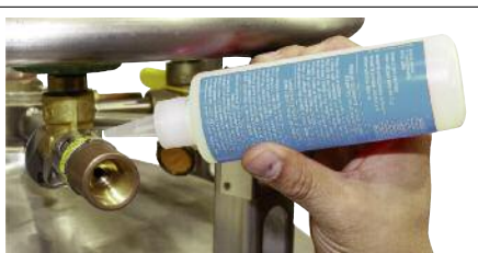
Oxygen Safe Valve Leak Check see page 9A-21 for more info
